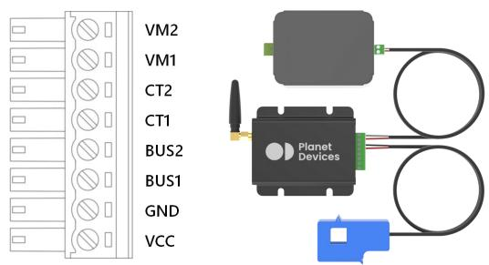
• VCC and GND are required to power an Atmo device
